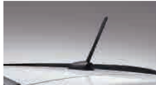
Roof-mounted pole antenna
