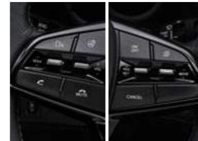
Remote control switches and cruise control system on the steering wheel
