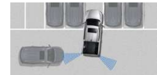
Rear Cross-Traffic Alert (RCTA) Assists the driver when backing up by detecting the presence of vehicles approaching on either side in the rear.
