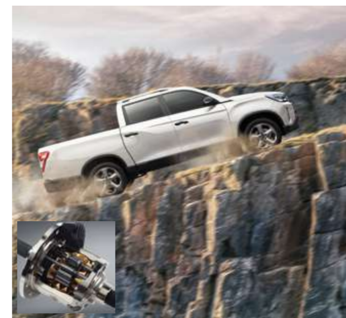
Locking differential On muddy or snowy surfaces, one wheel may slip or be lifted into the air. In this case, the locking differential forces both wheels on an axle to turn in unison, allowing the vehicle to recover its traction.
